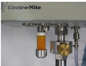
Figure 30: Pneumatic unit with tar filter block mounted next to the moisture filter
